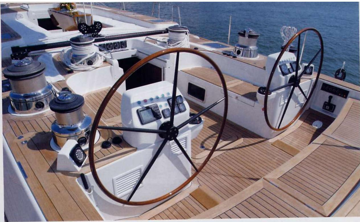
developed by Baltic. Fiberglass/Kevlar composite hull and deck entirely of carbon contain the weight so that equipment and systems could be positioned optimally, for maximum sailing comfort and performance. These qualities are guaranteed by a construction so light that the weight was easily kept within project estimates. Judel & Vrolijk (who designed "Alinghi", winner of the most recent
